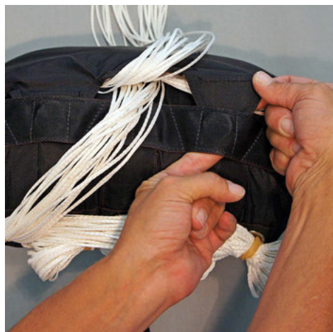
9. Tuck the stop tabs into the magnetic tab pockets.
