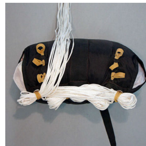
4. Top view stowing the top stows.
