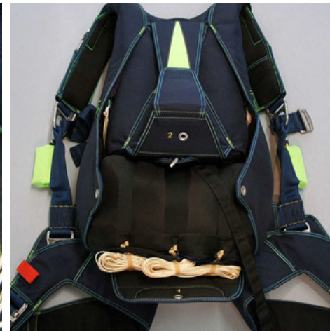
5. Place the main deployment bag in the pack tray with the lines facing down.
