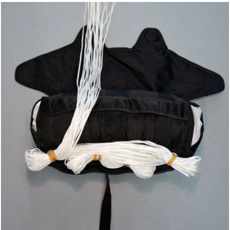
4. Top view of center and outside stows.
