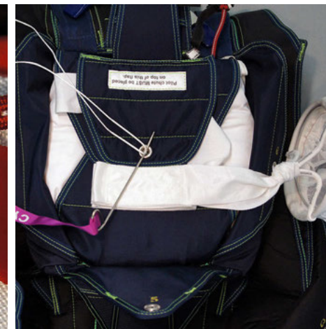
26. Close #2A cover flap and fold bridle crossways as shown.
