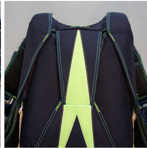
2. Close riser covers over the risers
