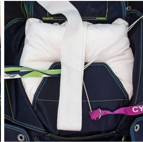
15. Close reserve #1 flap, then place bridle on top as shown.
