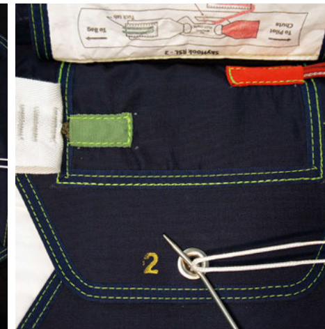
23. Insert the green loop into green tuck tab.
