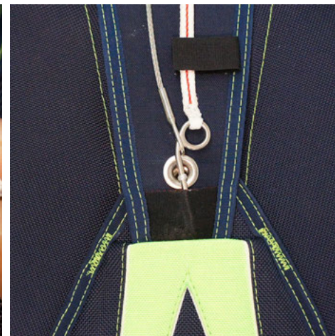
36. Insert the reserve pin through reserve closing loop and tuck it under the protector pocket.
