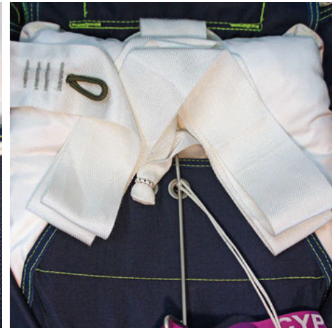
18. Fold bridle in "V" as shown.
