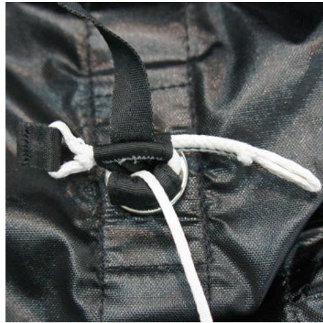
4. Pass the ALink through the through the bridle stow as shown.
