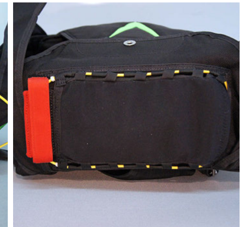
6. Thread yellow cable through loop under Type 12.
