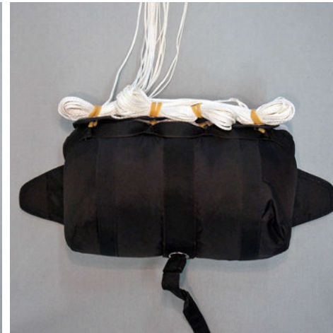
3. Stow the second center stow, then the two outside stows.
