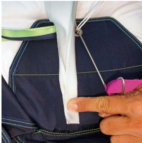
16. Tri-fold reserve bridle lengthwise.
