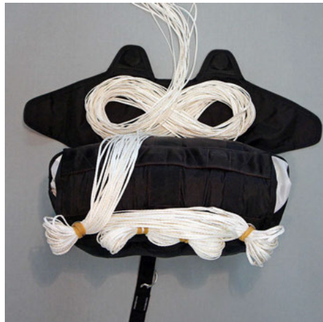
6. Neatly fold the suspension line in a figure of 8 as shown.
